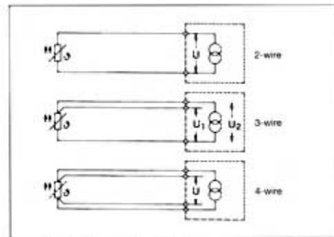
Fig. 21: Connection of resistance thermometers
