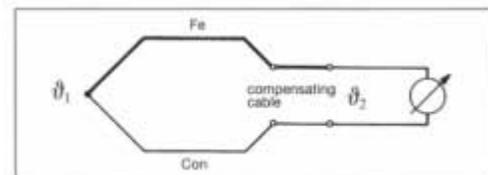
Fig.4: Thermocouple with compensating cable
