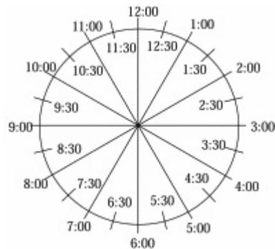
Holes should be located in degrees or clock time if possible, this will allow for the correct placement of holes. *Note: Every minute on the clock is 6°.*
