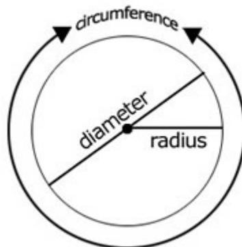
Hopefully, you can get this information from a drawing, but if not, you can refer to the above graphic and easily make your own measurement (We only need one of the dimensions from above). Next, determine the width of the heater and the length of the lead wire if appropriate.
